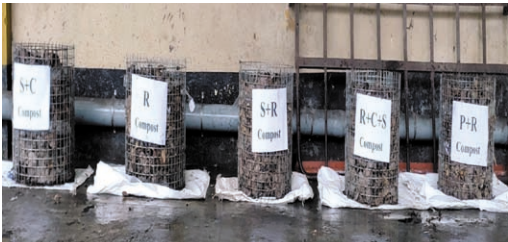
Fig. 1. Biobins set up for composting slaughter house waste
