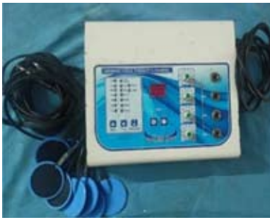
Fig. 1. Transcutaneous electrical nerve stimulator
