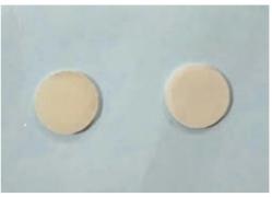
Fig-3 Prepared pellets of KBr and urolith for FTIR – ATR spectroscopy
