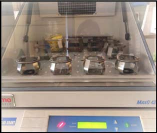
Fig.2. Decellularisation in a shaking incubator
